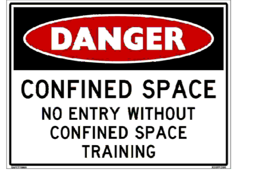
DETAIL - CONFINED SPACE SIGN NTS SIGNAGE TO BE AFFIXED BENEATH EACH ACCESS GRATE OF THE OSD TANK AND PUMP OUT TANK
